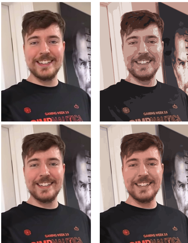
Fig. 4. Sample image 2. From top-right, clockwise, sample image compressed ( k=10 ), sample image compressed ( k=50 ), sample image compressed ( k=250 ), sample image original
